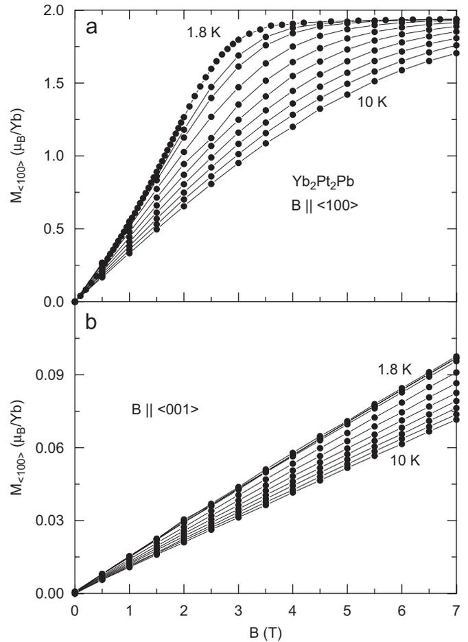
Fig. 2. The magnetic field dependence of (a)  $M_{(100)}$  and (b)  $M_{(001)}$  between 1.8 and 10 K for  $B\parallel\langle 100 \rangle$  and  $B\parallel\langle 001 \rangle$ , respectively.
